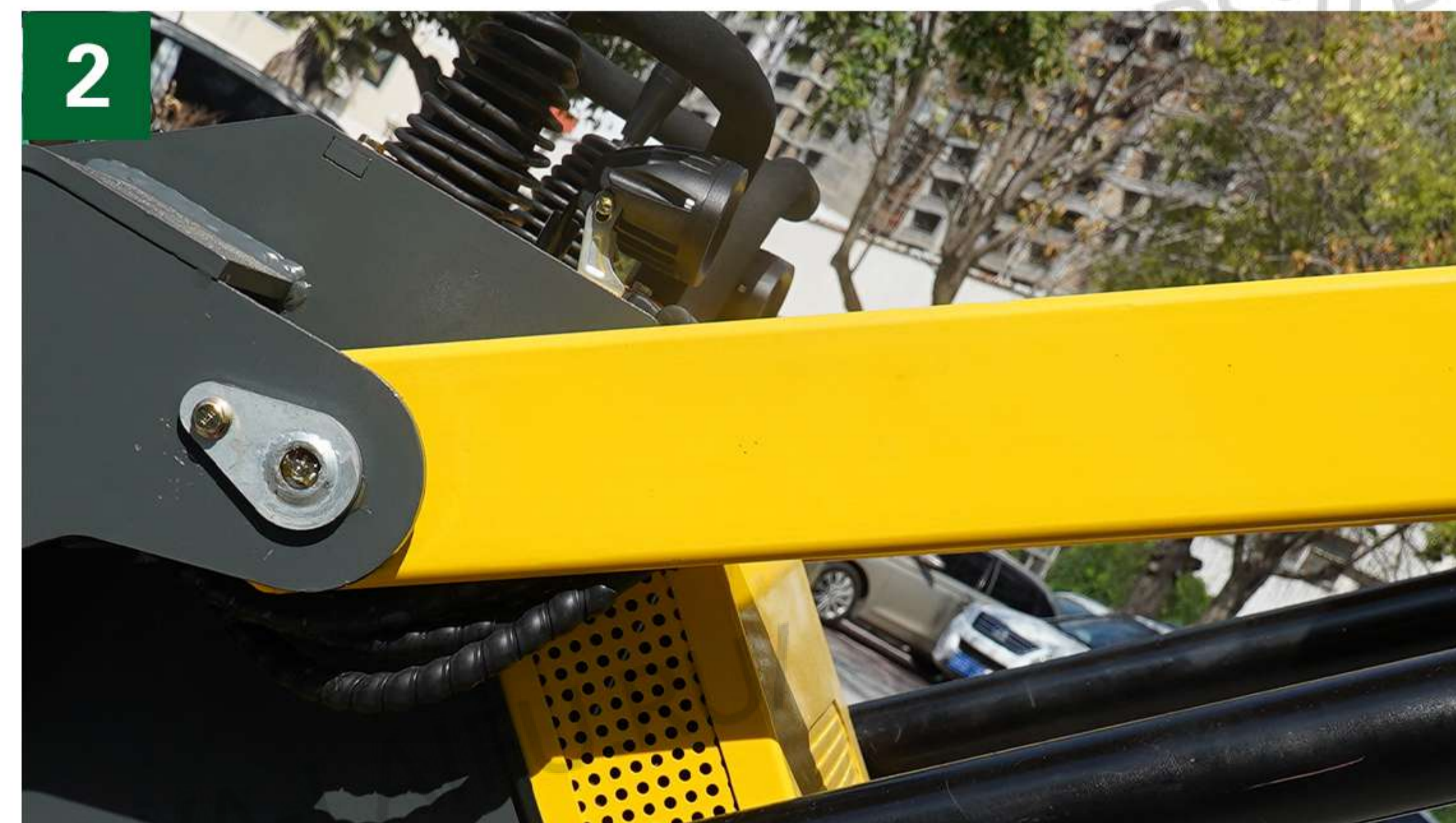
The oil pipe adopts a built-in pipe arrangement, which can effectively protect the oil pipe, reduce wear and tear and prolong the service life of the oil pipe.
