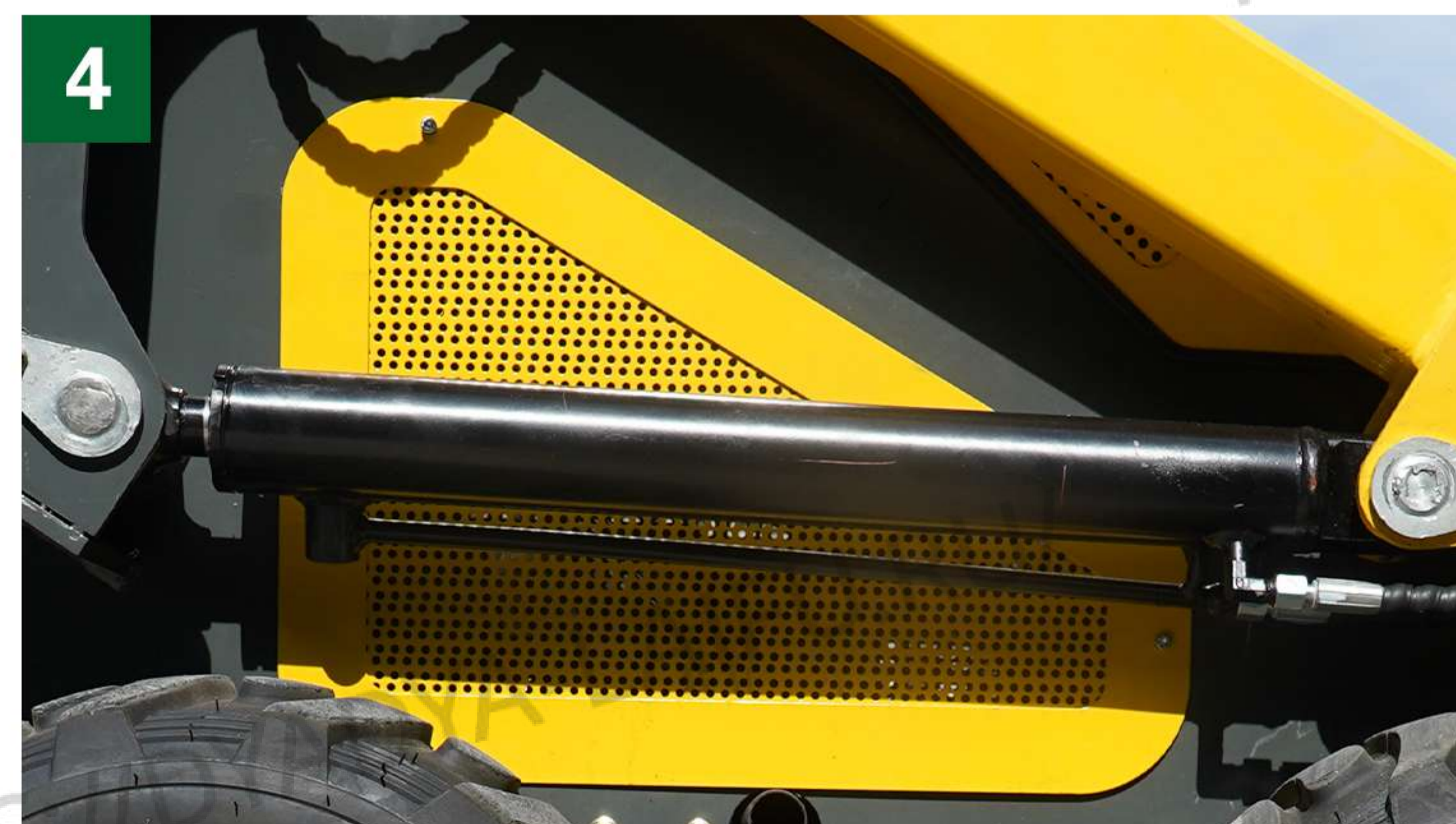
The inversion of the cylinder can effectively protect the cylinder rod from damage and prolong the service life of the cylinder.
