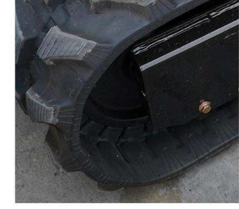
The guide wheel and tensioner can guide the direction and tighten the track.
