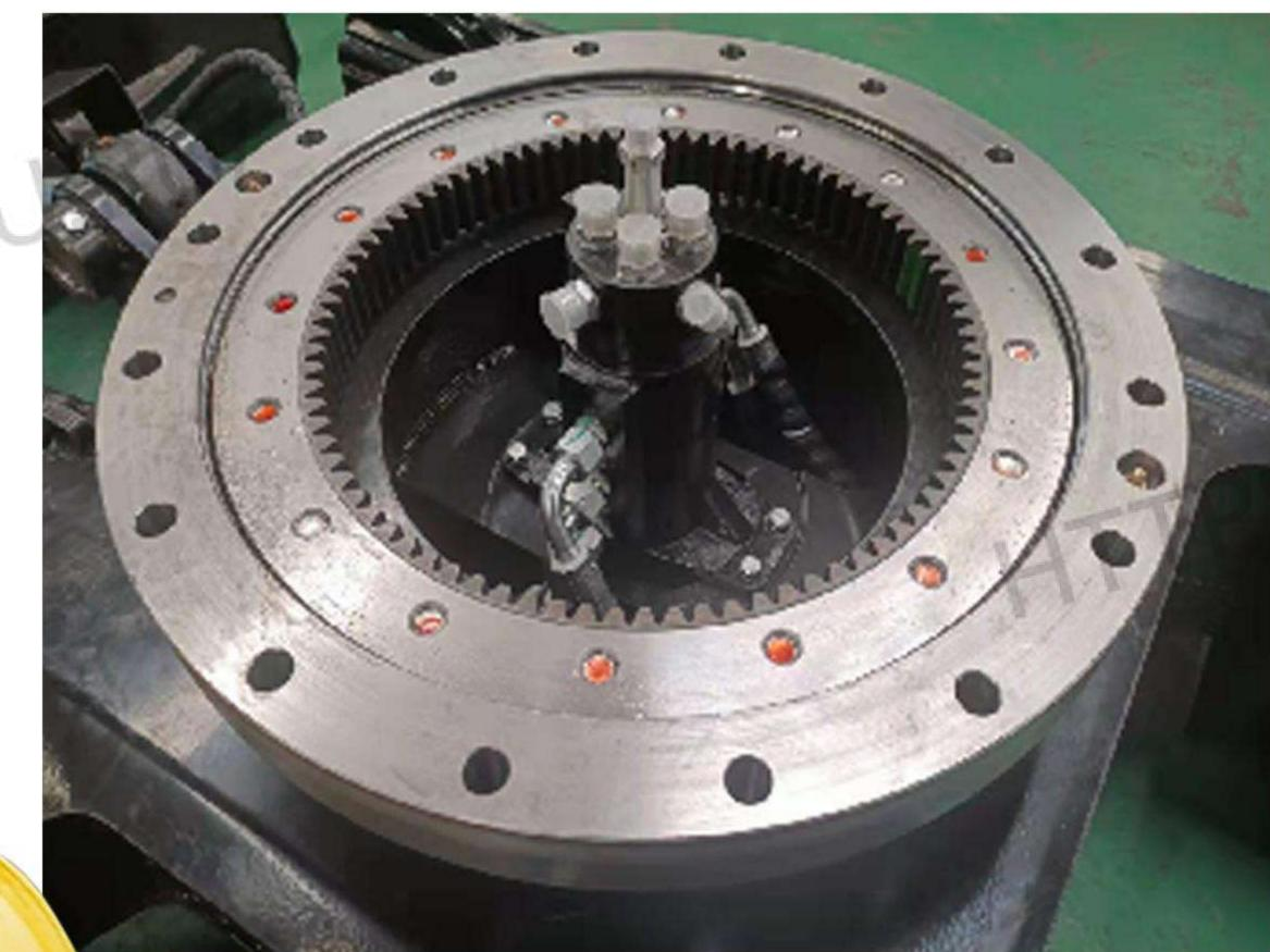
The tooth surface is quenched to greatly enhance the hardness of the tooth surface, improve the working strength and service life
