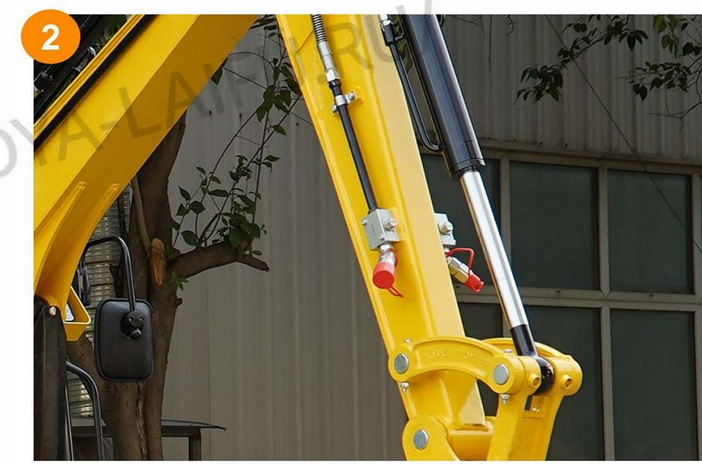
The breaker stop valve can effectively prevent oil leakage from the broken oil pipe when installing the breaker.
